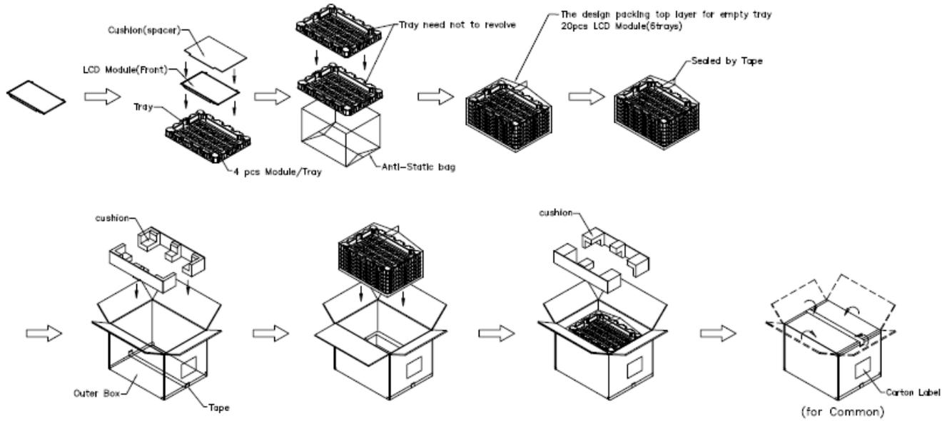
Figure. 7-2 Packing method
