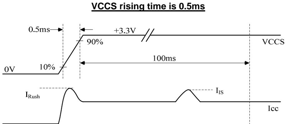
Note (3) The specified power supply current is under the conditions at VCCS = 3.3 V,  $T_a = 25 \pm 2 \text{ }^\circ\text{C}$ , DC Current and  $f_v = 60 \text{ Hz}$ , whereas a specified power dissipation check pattern is displayed.
