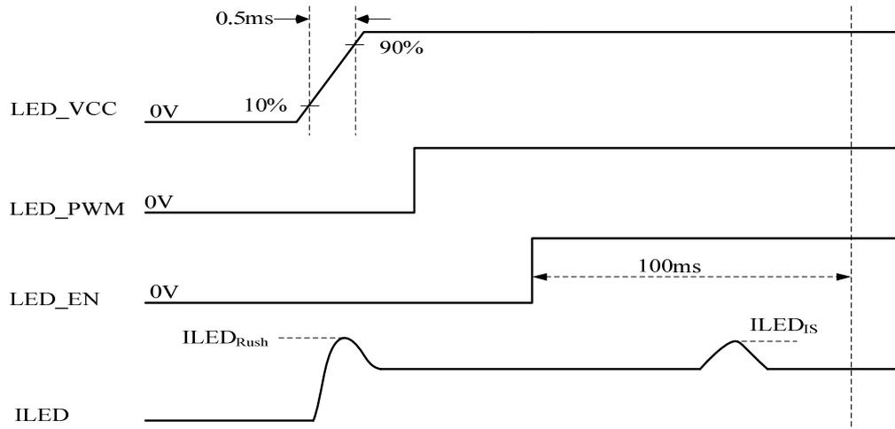
Note (2) If PWM control frequency is applied in the range less than 1KHz, the “waterfall” phenomenon on the screen may be found. To avoid the issue, it’s a suggestion that PWM control frequency should follow the criterion as below.
