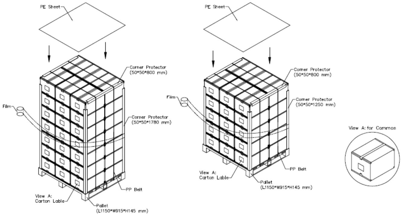
Figure. 7-3 Packing method
