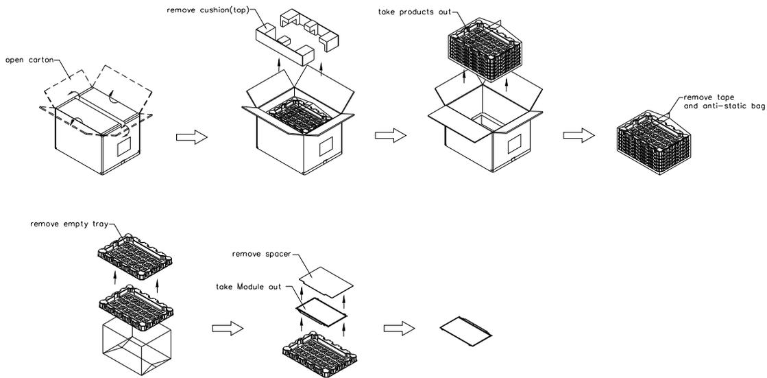
Figure. 7.4 un-packing method
