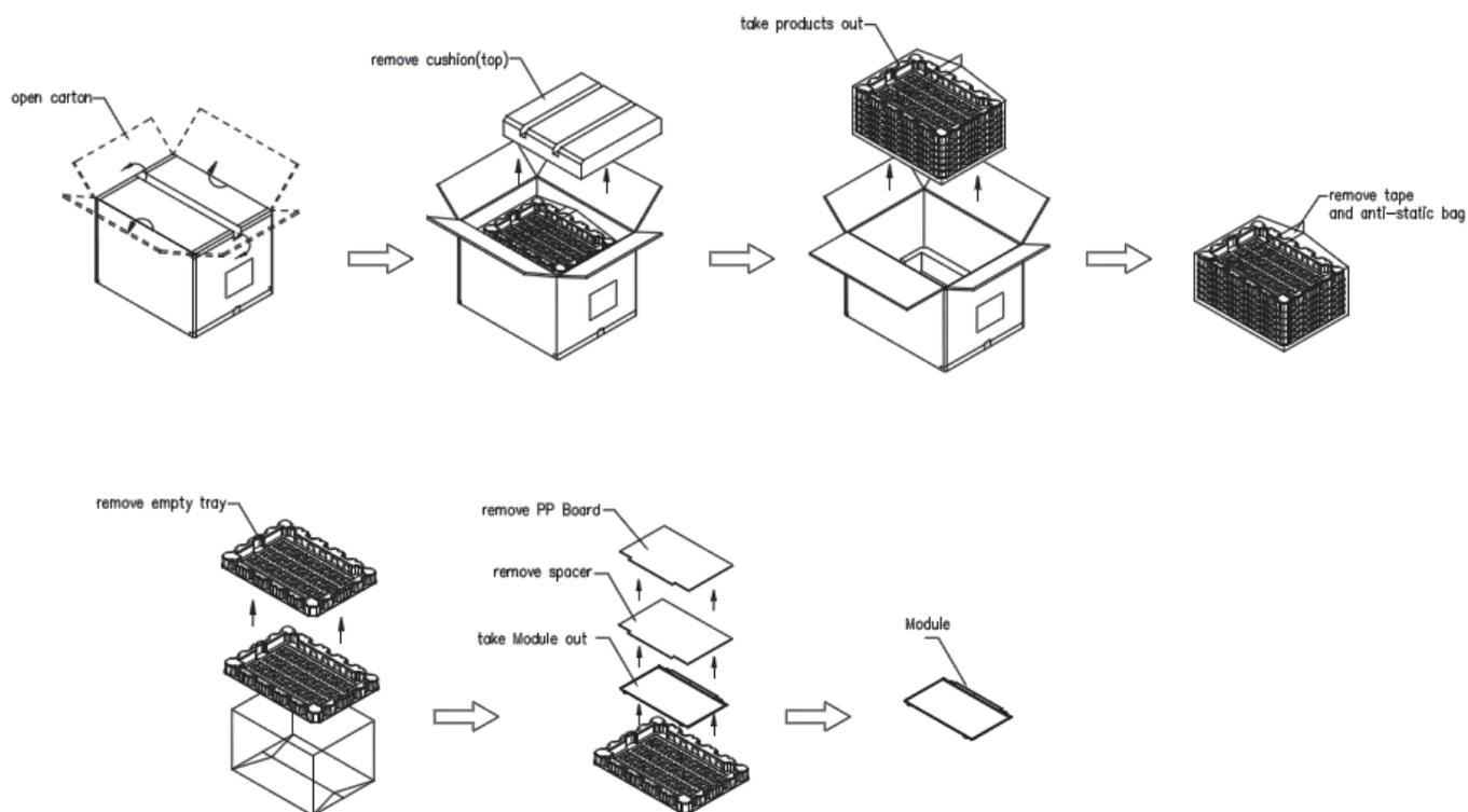
Figure. 7-3 Un-Packing method
